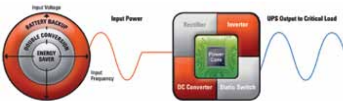
Input power quality out of rectifier tolerance
