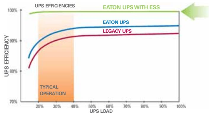
**ESS enables market-leading 99 percent efficiency** across the entire operating range. Compared to conventional 'eco-mode' capabilities available with legacy products, ESS offers the best possible efficiency and the fastest transition times to double conversion when power disturbances occur.
