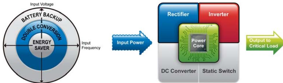
Figure 2. Active components engaged during double-conversion operation.
