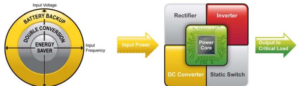
Figure 3. Active components engaged during battery backup.
